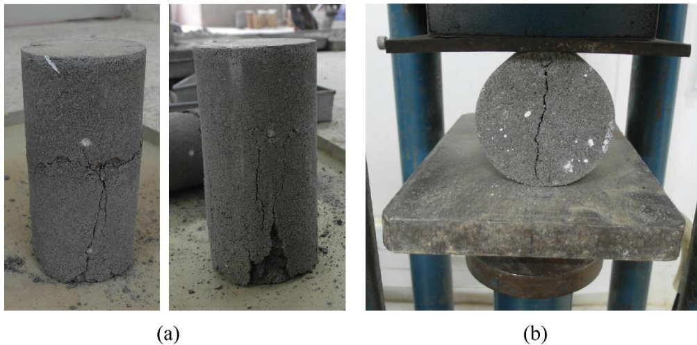
Figure 5.28 Failure patterns observed: (a) Compression test; (b) Tensile test.
