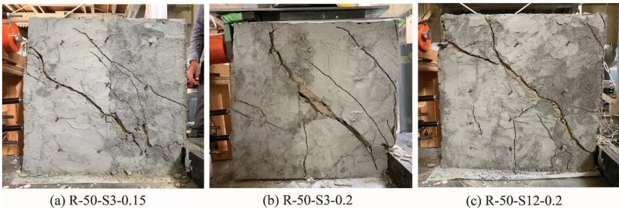
Figure 3.53 Final failure mode of RE walletes under in-plane shear loading.
