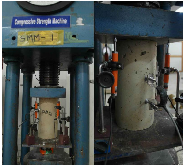
Figure 4.23 Test set up for material characterization of stabilized mud mortar.
