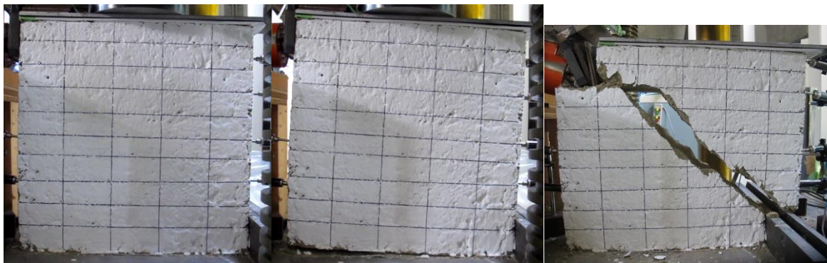
(a) At 5 kN (b) At 10 kN (c) At final failure
