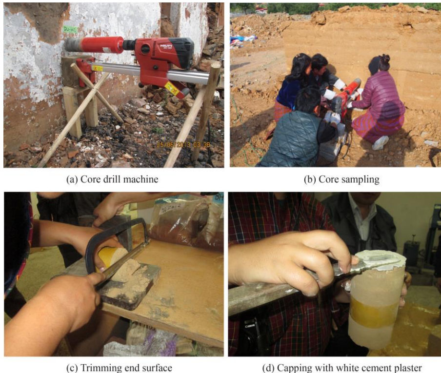
Figure 4.18 Sample collection for the material test.
