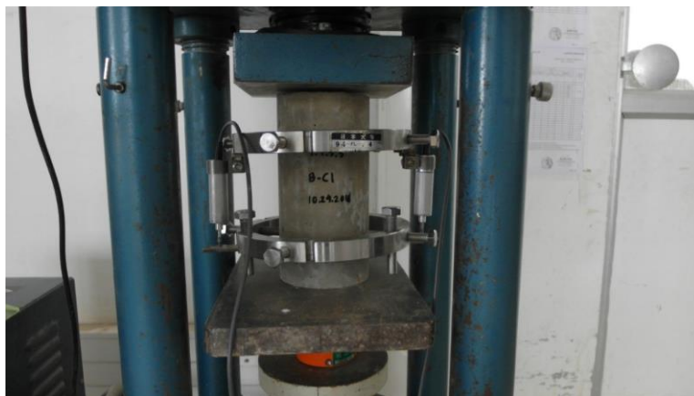
Figure 4.22 Test set up for material characterization of PCC.
