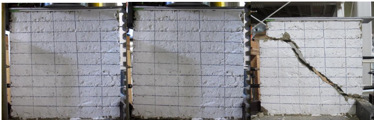
(a) At 5 kN (b) At 7.5 kN (c) At final failure
