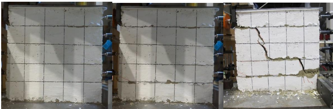
(a) At 2 kN (b) At 8.5kN (c) At final failure
